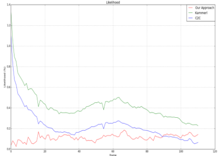
Figure 7. Likelihood of the distance error for every point in the trajectory with respect to its ground truth.
