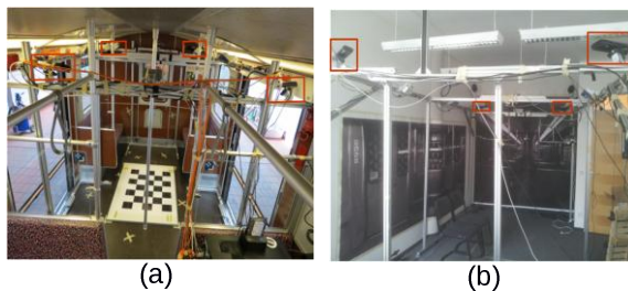
Figure 3. 3(a) Camera mounting configuration within the train wagon and 3(b) in the simulated environment.
