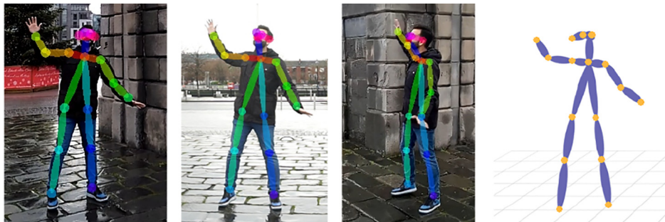
Fig. 4. Skeleton detected in several input images [38], and the final 3D reconstruction.
